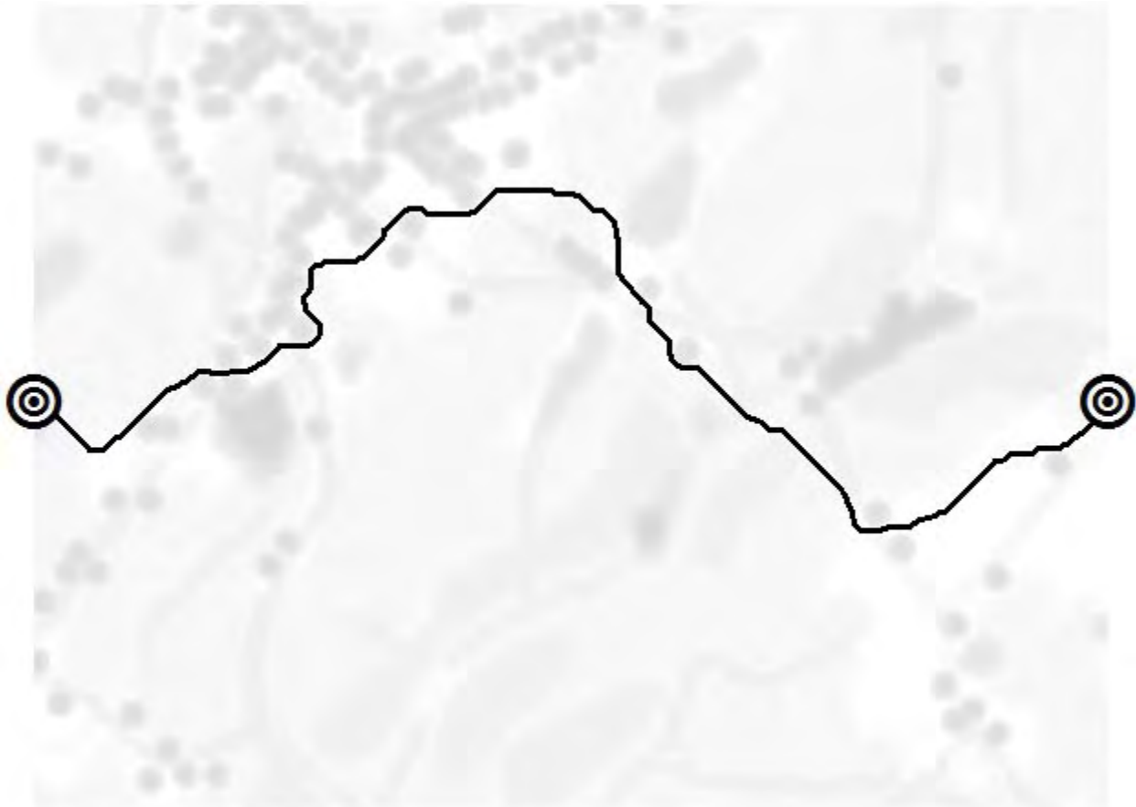
Fig. 2. The Centerline of Minimum Cost. The relative cost of traversing each location within a geographical area is indicated in gray, with darker shades corresponding to higher costs. The linear path in black connects the two termini depicted as concentric black circles with the lowest possible sum of those incremental costs.
