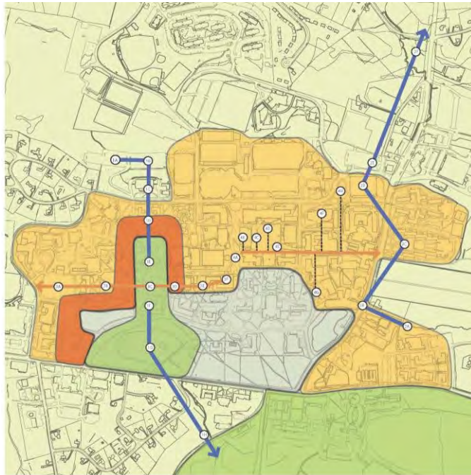
Figure 3 Masterplan diagram: central open space core, shifted density districts, stormwater treatment trains and pedestrian corridors.
