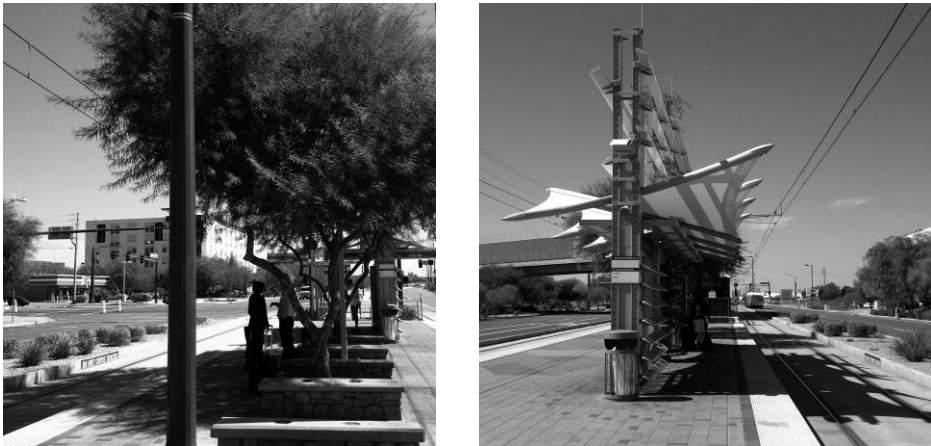
Figure 1 & 2. Side by side approaches to shade show trees and a manmade structure. The trees were found to be more effective in cooling the air and providing a comfortable sitting environment. (Phoenix, Arizona, photos: Lindhult)
