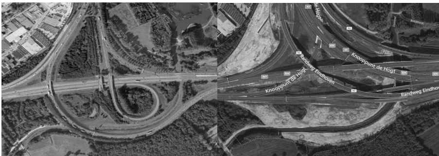
Figure 2. A2 Randweg Eindhoven – Dommeldal, in 2005 (left) and in 2009 (right) when former road space is given to the creek and broad viaducts are constructed (Sources: Google Earth and Bing Maps)
