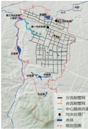
Figure7:existing Drainage System
