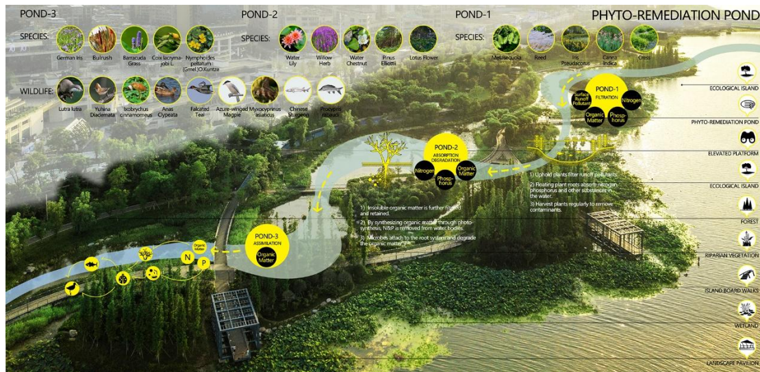
Figure 7: Phyto-remediation System, a Functional Landscape—Resilient design considerations uses materials that would survive flood even if totally submerged by water.
