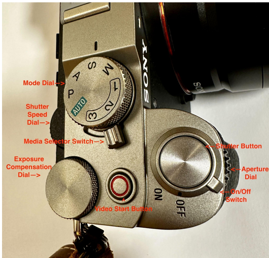
Figure 11—The placement of the dials, switches, and buttons allow for separation of controls; the sides of the two dials vary in texture; engraved into the top of the two dials and the shutter button are very fine concentric lines that resemble the fingertip’s fingerprint; the only surface on the camera
