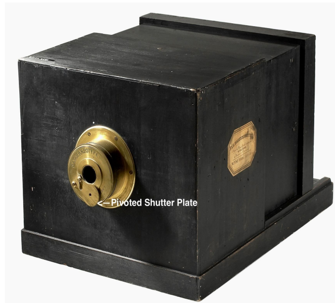
Figure 1—1839 example of a Susse Frère Daguerreotype camera; note the metal pivoted shutter plate that allows light into the lens. (Photo by Luidmila & Nelson, Susse Frère Daguerreotype camera 1839, August 5, 2010, Wikimedia Commons).
