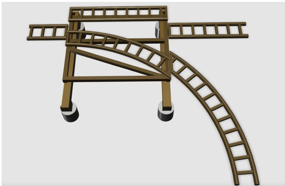
Figure 5 - Switch Track Diagram, HMA (Credit: AmusementLabs)
