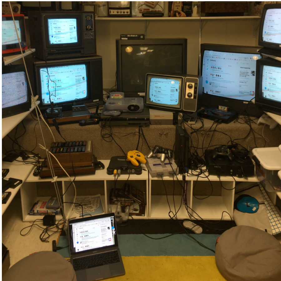
Figure 7 – Documentation of a Media Archaeology Lab's experiment showing Lori Emerson's Twitter feed transmitted over VHF radio to 8 analog televisions.
