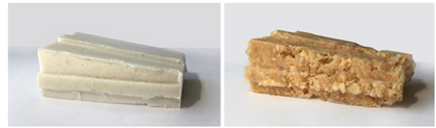
Figure 3. Compressive blocks of eggshell and agar agar (left) and sawdust and agar agar (right) in preliminary wedge-shape form with interlocking key.
