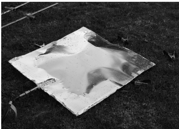
Fig. 5. Ravioli during hydro-forming (photo credit: Bennett Mueller)
