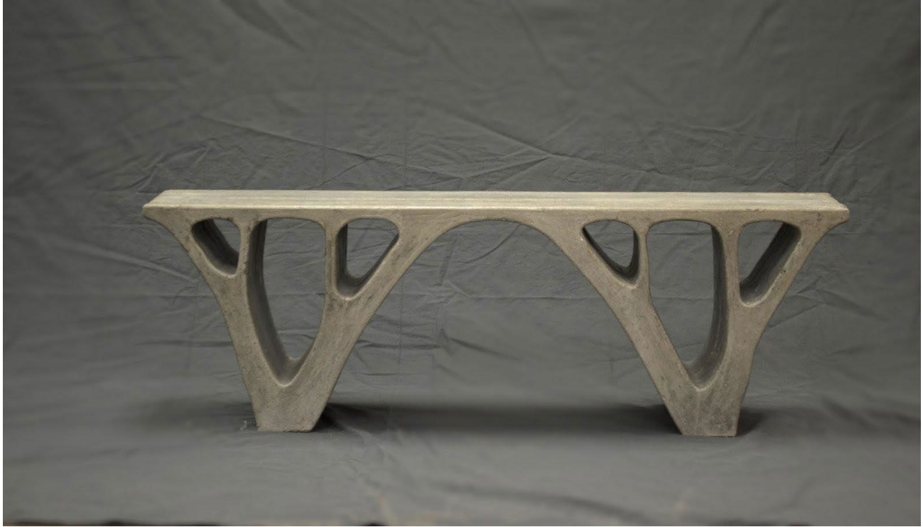
Fig. 6 Photograph of cast beam. Overall dimensions: 50" (length) x 10" (width) x 16" (depth); weight: 206 lbs
