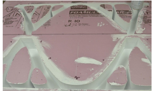
Fig. 5 Image of CNC-milled polystyrene casting form
