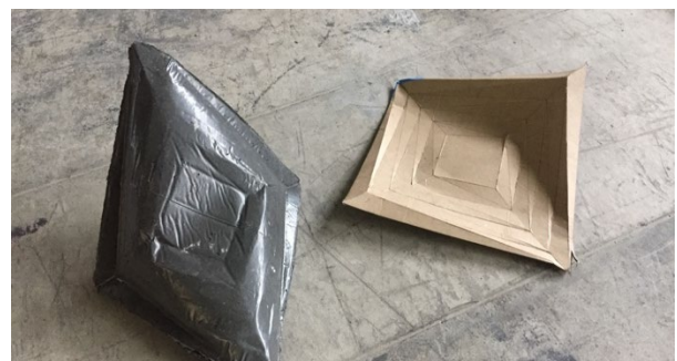
Fig. 3. First simple cardboard formwork and cast.
