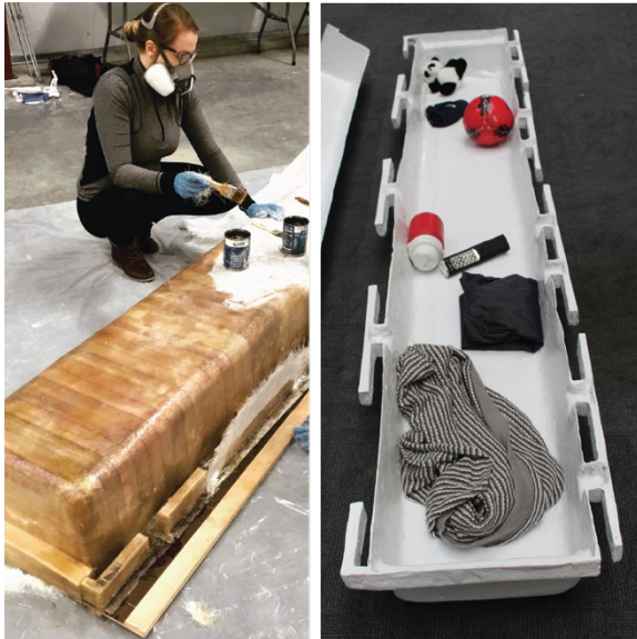
Fig. 1. Constructing fiberglass bin for Store Floor design, 2017
