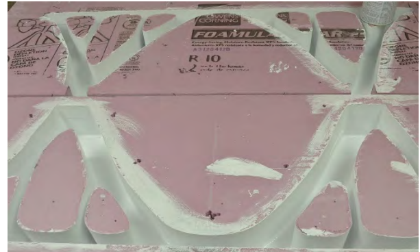
Fig. 5 Image of CNC-milled polystyrene casting form
