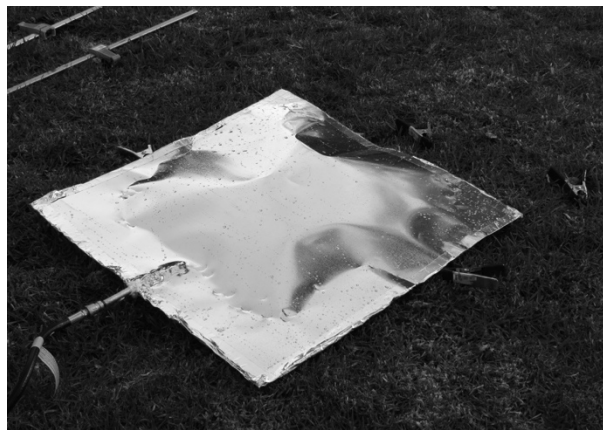
Fig. 5. Ravioli during hydro-forming (photo credit: Bennett Mueller)
