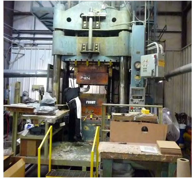
Figure 3 | Large press for compression molding thermoset plastics. Penn Compression Molding is a CM and focused on manufacturing with thermoset plastics.
