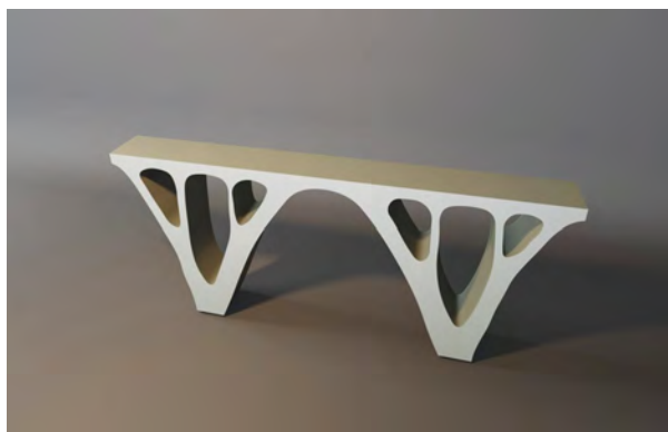
Fig. 3 Rendering of optimized topology chosen for fabrication
