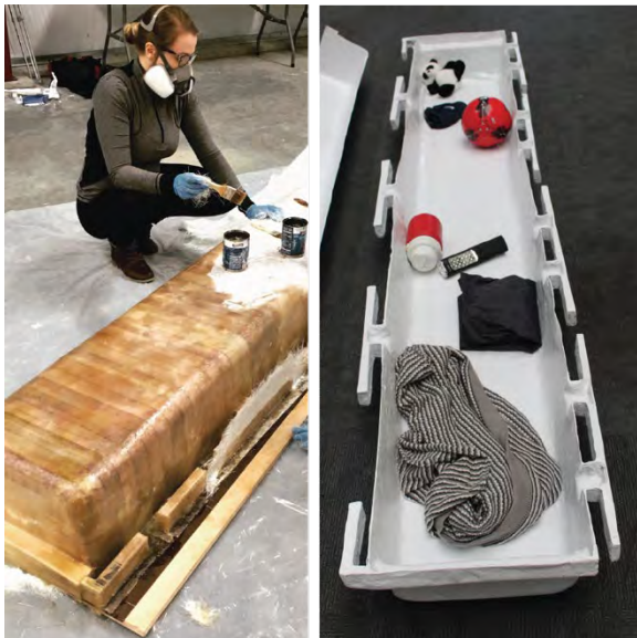
Fig. 1. Constructing fiberglass bin for Store Floor design, 2017
