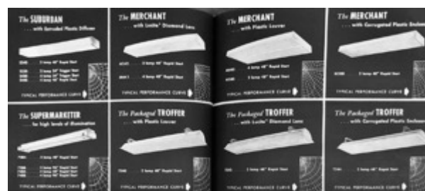
Fig. 4. The combination of easily extruded and molded plastic with the linear, diffuse nature of fluorescent lighting led to new fixture types that could be easily matched to the needs of new, open plan offices. Miller Company advertisement, Architectural Record , May, 1955. xi.
