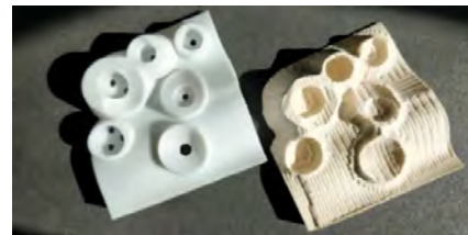
Fig. 4. Surface studies of 3D printing versus CNC milling developed by Amir Hussain, Bristie Smith & Jeremy Gremillion
