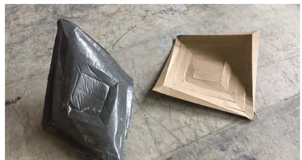
Fig. 3. First simple cardboard formwork and cast.
