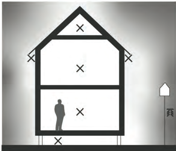
Fig. 1. Sensor placement diagram, section cut east/west.
