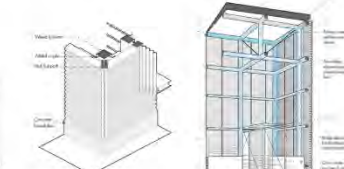
Figure 16. Floor Slab Break Section Showing the structure of the floor slabs and how they relate to the corner.
