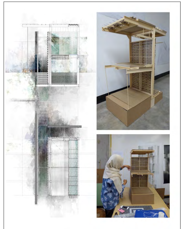
Figure 3. Drawings and 1'=1'-0' scale physical models studying structural systems in their design work. (Anggitta Nasution-Zurman, Fall 2015)
