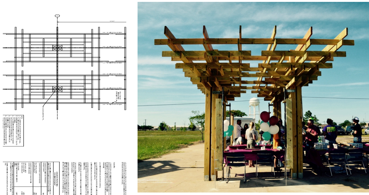
Figure 2: Farmers Market Structural Framing Plan, and a view after the prototype completion
