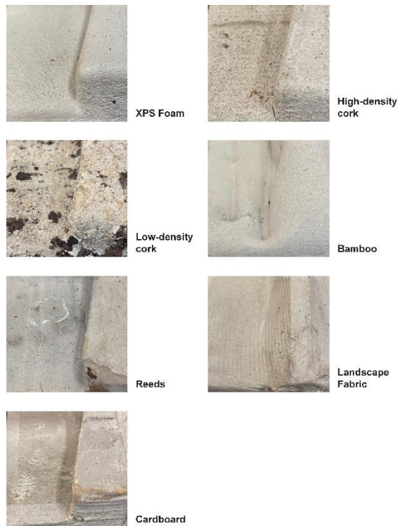
Fig. 8. Photographic comparison of cast beam texture, characterized by formwork material difference.
