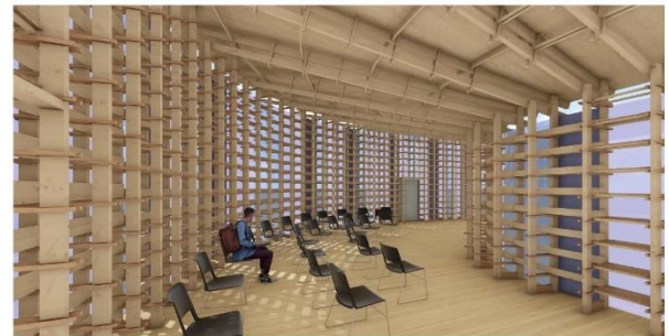
Fig. 2. The first prototype developed by Team 1. Curved beams are used in the roof system. Source: Nicholas Frantzeskos, Christina Donabella, Alexa Cutruzulla
