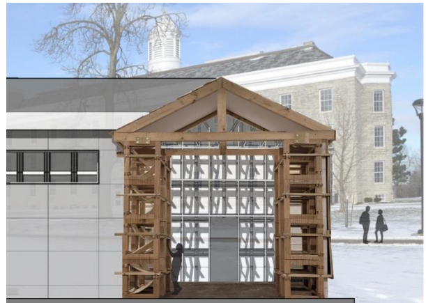
Fig. 6. Team 2 developed their first prototype with a space frame wall system. Source: Emily Connor Vollo, McCormick, and Jacob Maciejewski
