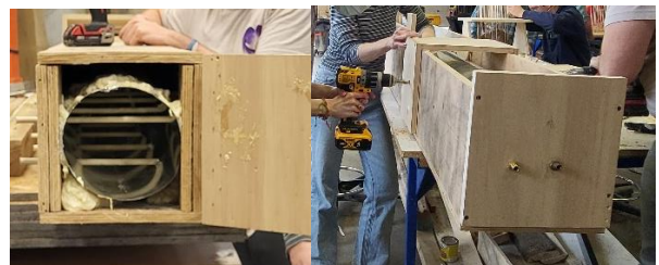
Fig. 3. Team 1 made a wood steam box and used it for curving ash wood elements.
