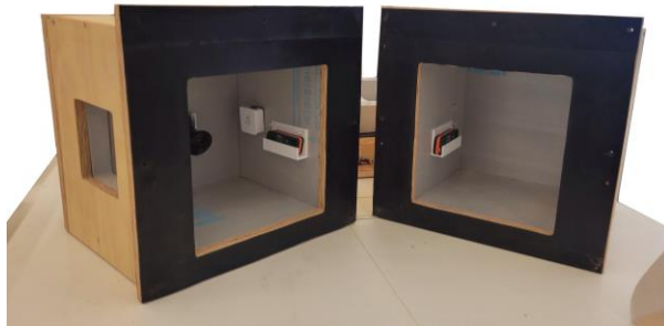
Fig. 2. Interior of hotbox chambers.
