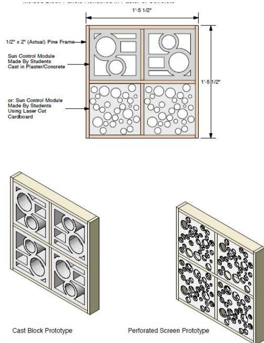
The fabrication and design phase spanned three weeks, during which students gained hands-on experience with various materials and techniques. In the shop, students worked with plasters to create vacuum-formed molds and cast plaster units. Using templates provided by the professors, students assembled four units into a screen
