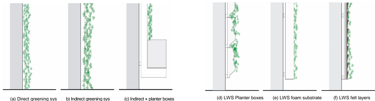
Figure 2: Prototypes of vertical greening systems evaluated by LCA study (Ottele et al, 2011)
