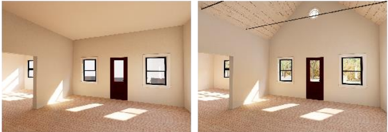
Fig. 9. Renderings showing the Fire House with a cold roof and flat ceiling (L) and hot roof with vaulted ceiling (R)
