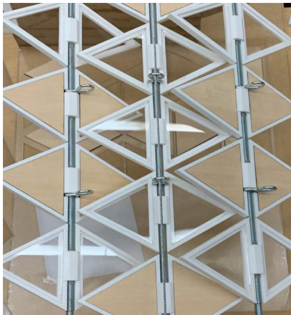
Fig. 2. Student Prototype: Threaded Rods, 3D Printed Frames, Wood, and Acrylic Spanning Structure
