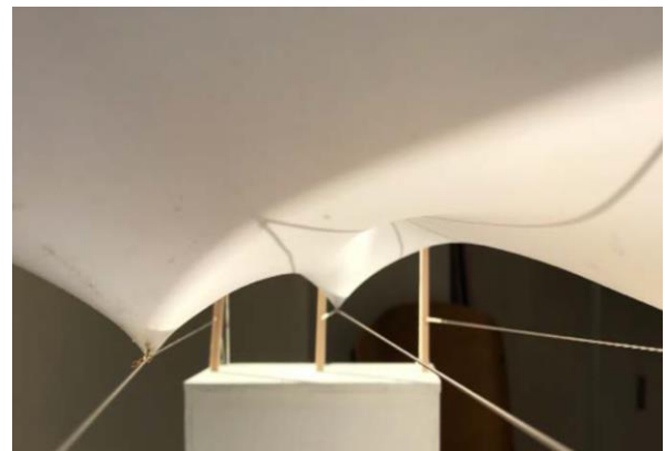
Fig. 4. Student Prototypes: Lycra and Nylon Wire Tensegrity Spanning Structure
