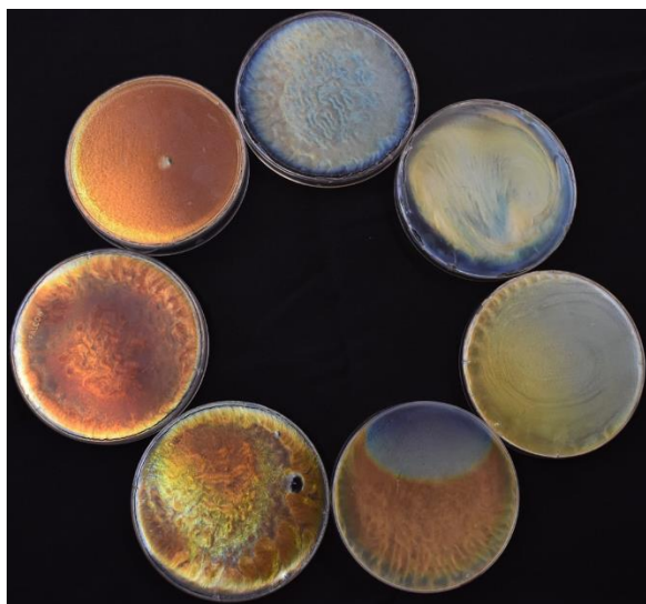
Fig. 8. Examples of iridescent colors obtained by combining CNCs and additives such as PEG.
