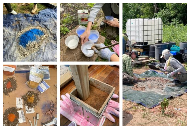
Image 4. Rammed-earth color testing and experimentation—including premixing dyes into the soil mixture and adding them to the sealant—to achieve the highest contrast for sign language visibility and bold colors.
