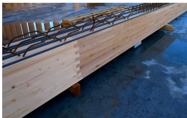
Fig. 2. Ash and Spruce Joint. Photo Credit: S. Jacob-Freitag (See European Standard EN 14080 for GL strength classes)
