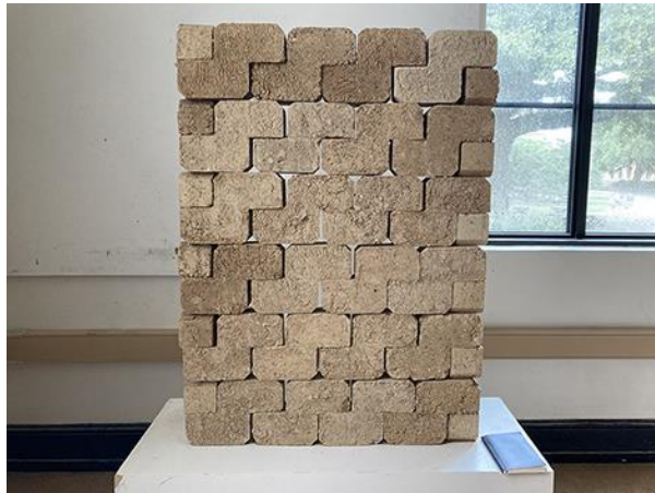
Fig. 9. Duck shape earth block wall assembly.
