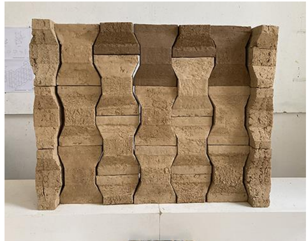
Fig. 11. Bow Tie shape earth block wall assembly.
