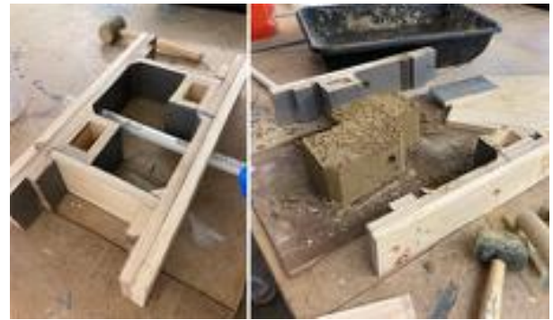
Fig. 8. Duck shape earth block fabrication.
