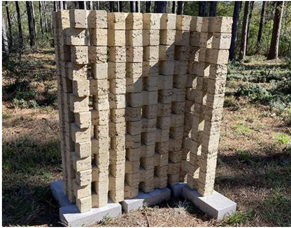
Fig. 7. H shape earth block wall assembly.
