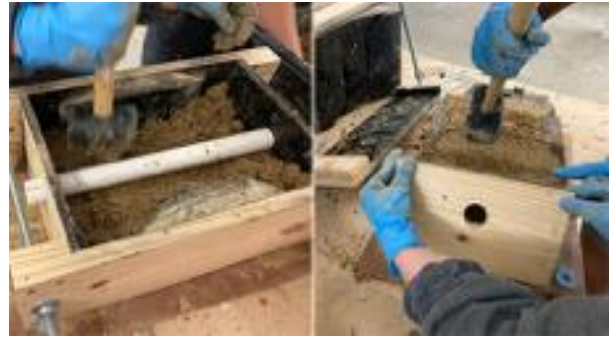
Fig. 10. Bow Tie shape earth block fabrication.
