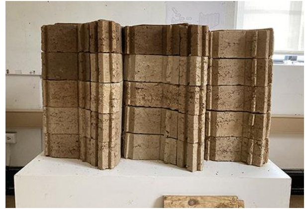
Fig. 13. Zig Zag shape earth block wall assembly.
