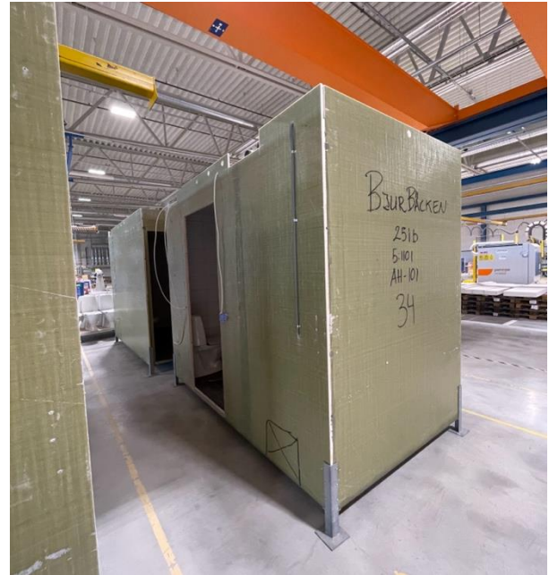
Fig. 5. Packaged Bathroom systems. Image by Author. 2024
