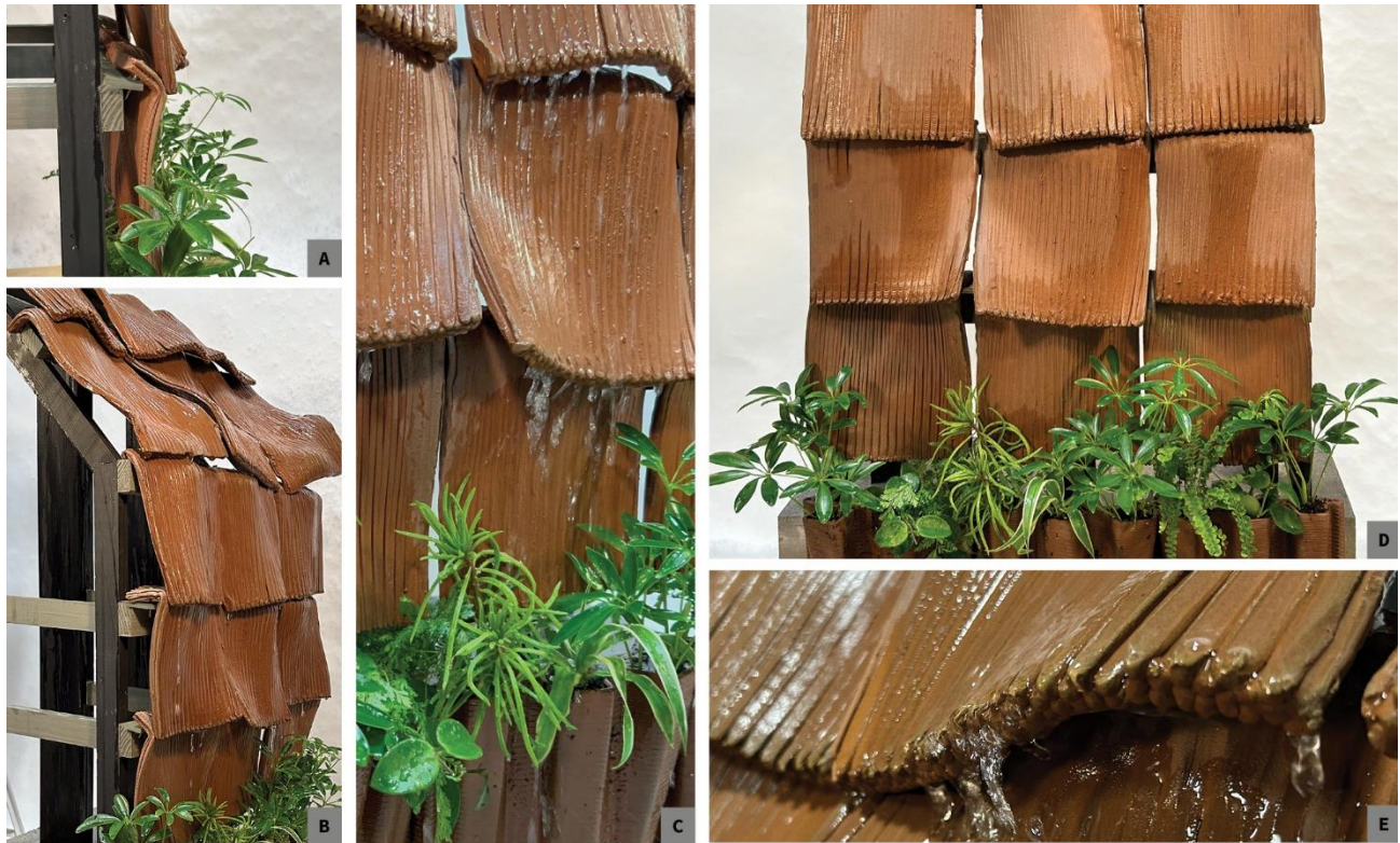
Fig. 7 (A) close-up of the tile attachment. (B) side view of the entire assembly. (C) water moving across the tiles. (D) front view of the tiles as they dry. (E) close image of the water passing over the tiles.
