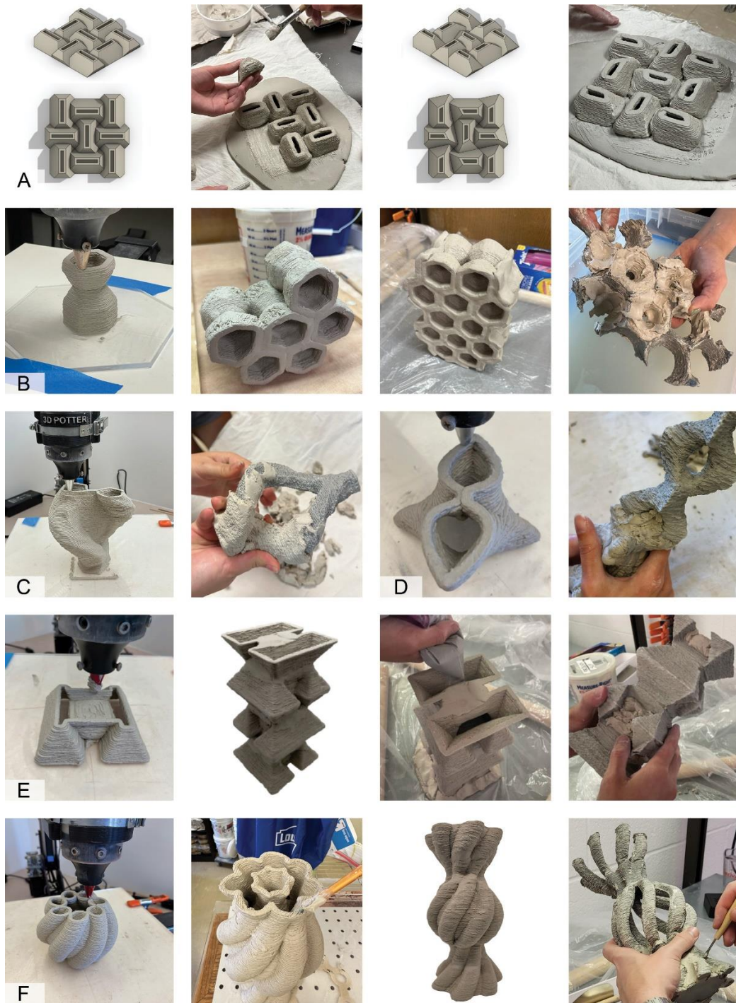
Fig. 3. (A) and (B) Assignment 1 focused on exploring modular clay formwork systems, serving as an introduction to clay 3D printing, hand-building, casting, and digital fabrication workflows. Team (A) utilized various tessellating forms to create tiles, while Team (B) employed an hourglass prismatic figure for double-sided formwork. (C-F) Examples from Assignments 2-4 investigate columns with openings. (C) and (D) examined closed toolpaths to create voids and open toolpaths for the casting material for Assignment 2. (E) and (F) showcased more complex designs incorporating various prints and hand-building techniques, building on skills learned from Assignments 1 and 2.
