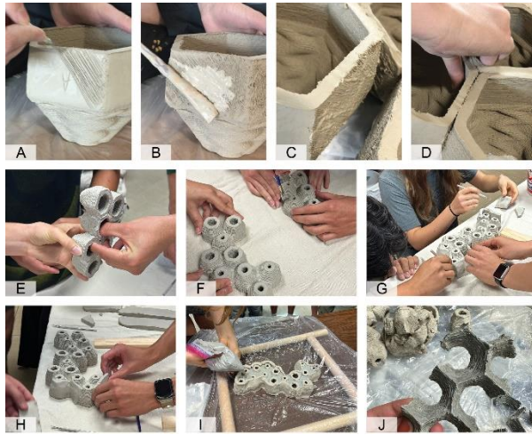
Fig. 2. Unit joinery process: (A) scratching of the lower half, (B) applying the liquid clay to the surface, (C) aligning the correct sides, (D) applying pressure to weld units. (E-F) Students learning how to create and cast hand-built paper clay formwork in an in-class workshop with pre-printed units.
