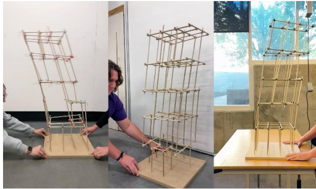
Fig. 1. Dynamic testing of push and pull physical models.
