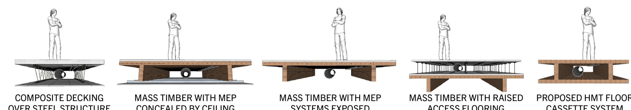
Each HMT cassette consists of two 3-ply CLT flanges and two glulam web members. Designed for spans up to 40 feet, the system reduces the need for interior bearing points. The cavities are designed to meet fire compartmentalization requirements and can be used for the passage of MEP systems, with top-down access provided at periodic hatches. A variety of flange-to-web connection methods were explored to ensure both structural integrity and ease of disassembly.
