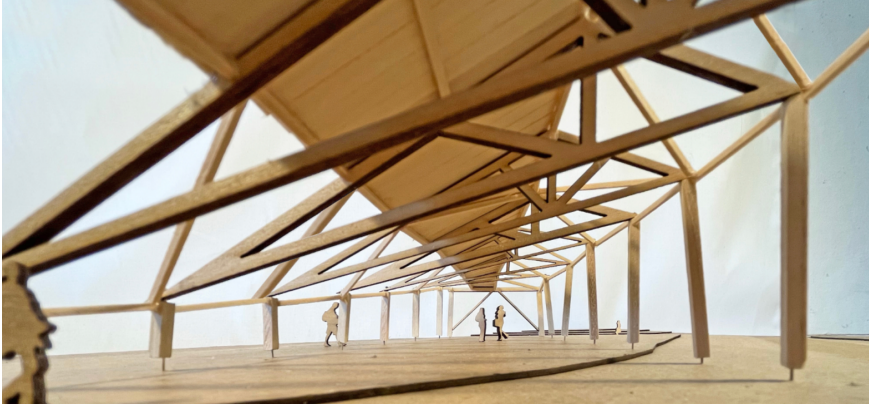
Figure 5: Column base elevated above grade, modeled to behave like a pin. Student work by Alice Clements and Shannon Rooney.
