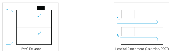
Figure 8: Diagram of modern air conditioning and diagram of Escombe natural ventilation. Source: (Garceau, 2022).
