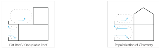
Figure 5: Diagram of flat roof with occupiable space and diagram of a typical sanatorium. Source: (Garceau, 2022).
