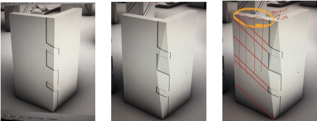
Figure 4: Screenshot images of a digital model were exchanged digitally, allowing team members to draw on top of the images and suggest new design potentials. These images specifically show the progression of the joint condition including diagonal notch, facet, and idea for faces.
