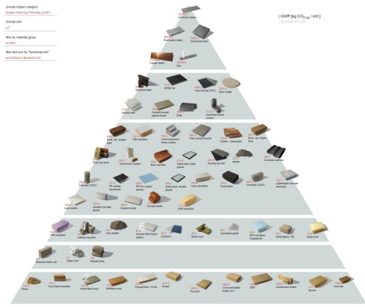
Figure 2: The Construction Material Pyramid. (CINARK 2023); and environmental impact calculation of Norvento Headquarters's wall using the Construction Material Pyramid. (Student: Libby Couture 2022)
