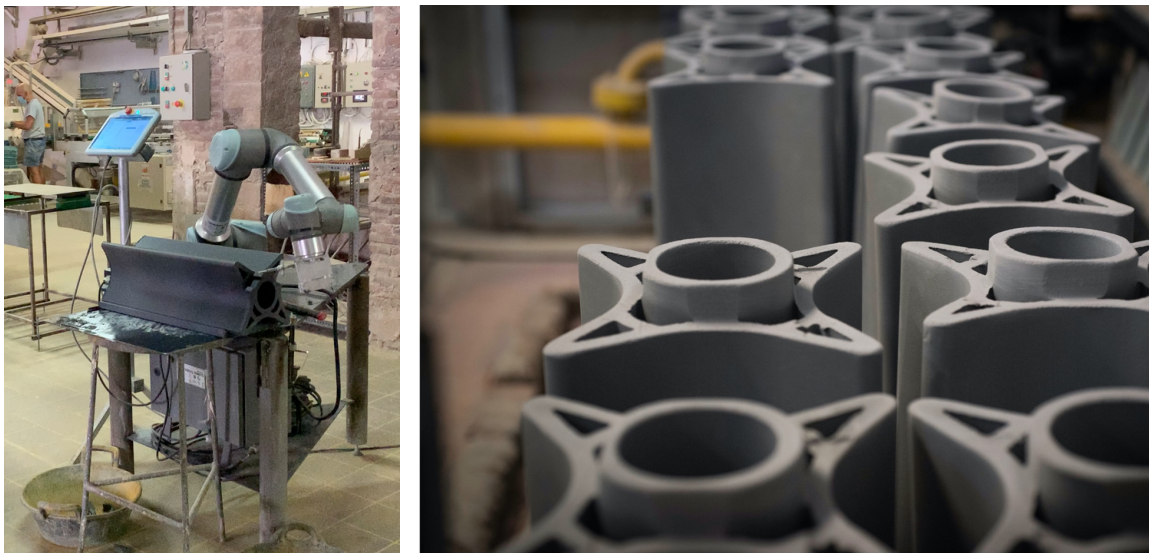
Figure 3: Hollow ceramic piece “Star” by Juan José Castellón, manufactured by Ceràmica Cumella. Left: robotic arm producing the interlocking connections / right: final pieces. Source: (Frau Recerques Audiovisuals 2021).
