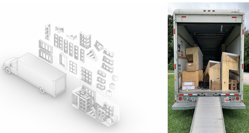
Figure 4: The installation was designed to fit within a single 26-foot-long U-Haul truck. Source: Authors; and photograph of the installation loaded for transportation. Source: Authors
