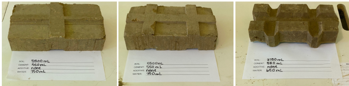
Figure 3: Geometric refinements: single cross, double cross, double cross & edge. Source: (Author 2020)
