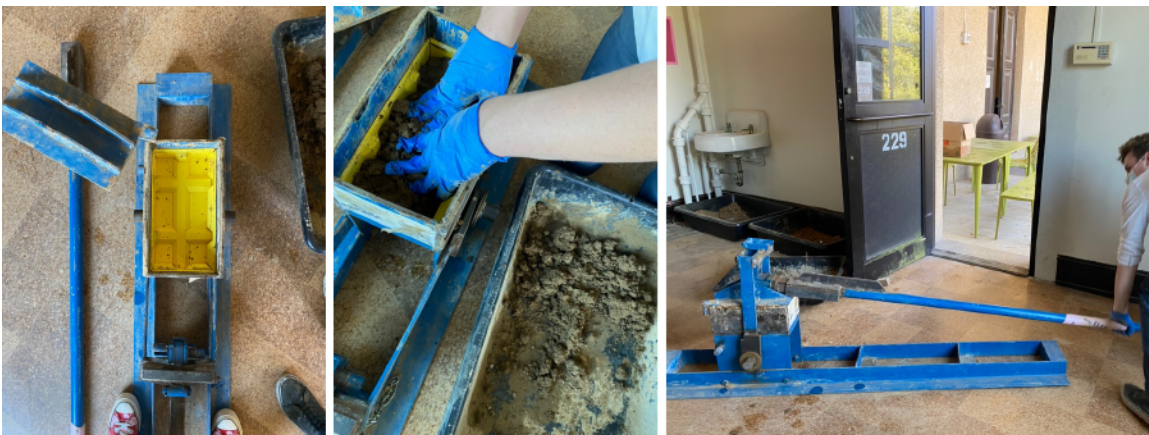
Figure 2: Compression chamber with insert, adding the earth mixture, and compressing the block. Source: (Author 2020)
