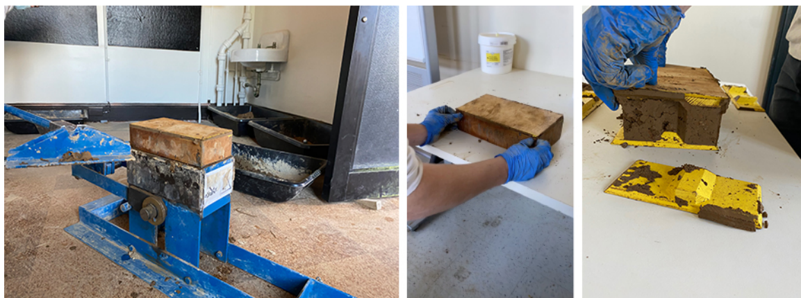
Figure 4: Removing the insert from the press and unmolding the block. Source: (Author 2020)
