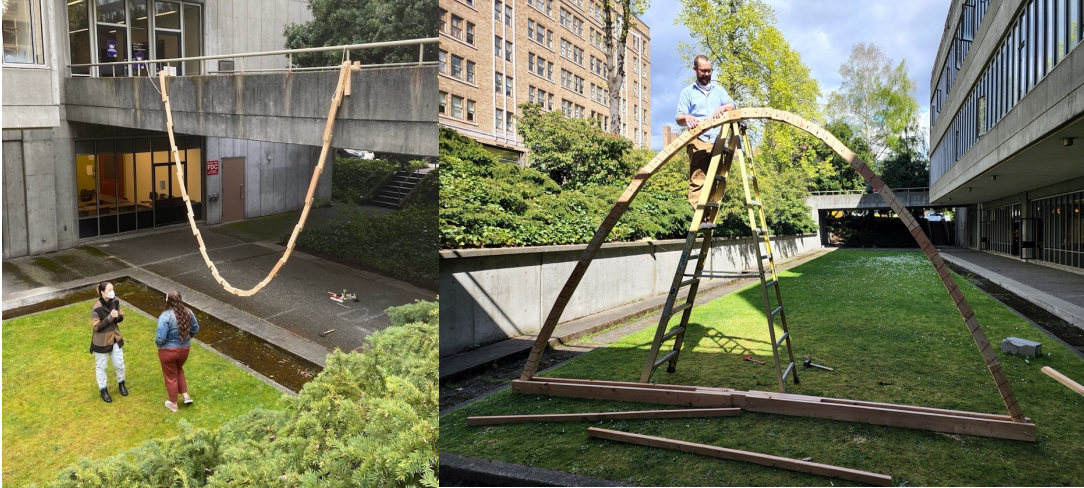
Figure 6: Hanging Chain to Standing Arch, Assembly. Source: (Tyler Sprague, Stephanie Cote 2022)
