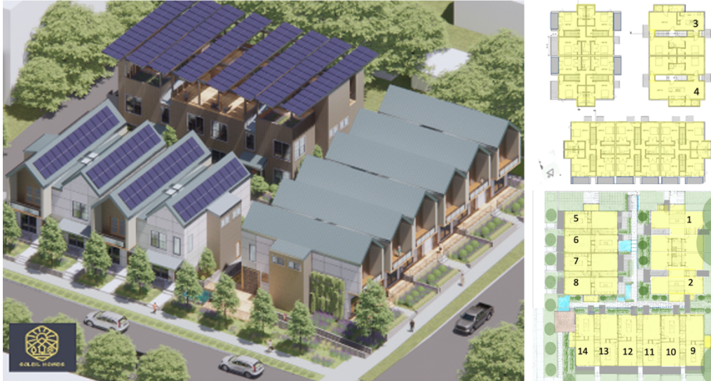
Figure 1: SOLEIL 14-unit middle density housing model proposed for a ½ block housing density transition zone. Source: (Garrison 2021)
