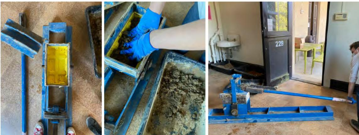
Figure 2: Compression chamber with insert, adding the earth mixture, and compressing the block. Source: (Author 2020)
