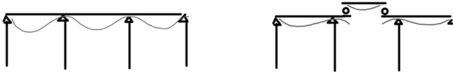
Figure 4: Class example of a continuous beam (indeterminate, left) transformed into a 3-part compound beam (determinate, right) that became a more common discussion in projects with the introduction of determinacy as a constraint.
