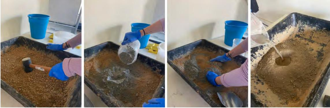
Figure 1: Multi step process to prepare the earth mixture for block fabrication. Source: (Author 2020)
