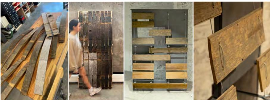
Figure 9: Wooden screen system using reclaimed wood. (Student: Anna Hartley and Jada Rezac 2022)
