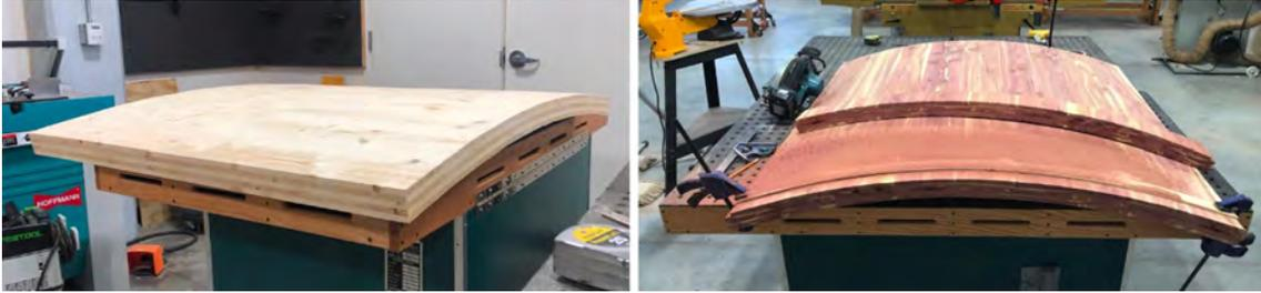
Figure 4: Post vac-formed lay-ups - XX-LAM Studio
