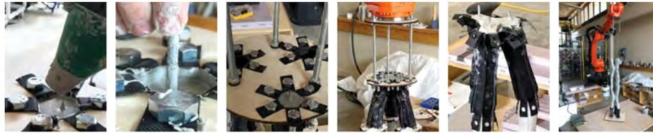
Figure 4: This image shows the process of pouring Rockite (A), placing all thread reinforcement immediately after casting (B), and leaving the material to cure (C). The bottom images represent the casting of the layers using the robotic arm (D and E) and the final column design without the base and the bottom formwork removed (F). Work by Mohammad Karkoutly. Source: (Mohammad Karkoutly 2022)
