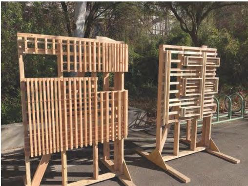
Figure 11: Cladding-Layering Iteration 2 examples, one with screws creating an ordering system, one without visible screws. Source: (Author 2022)
